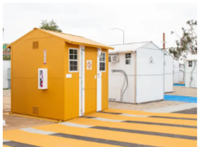
Micro-shelter – typically under 200 sqft - no kitchen or bathroom – not a dwelling unit, but is habitable space
